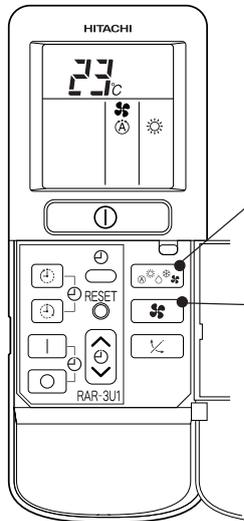
**1** Press the FUNCTION selector so that the display indicates ☀ (HEAT).
