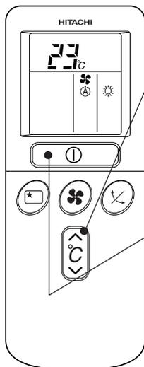
**3** Set the desired room temperature with the TEMPERATURE buttons (the display indicates the setting).
