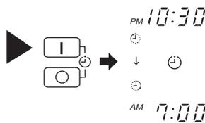
Example: For heating, the device will turn off at 10:30 p.m., and then turn on early so that the preset temperature be almost reached at 7:00 a.m.; for cooling and dehumidifying, it will simply turned on at 7:00 a.m. The settings of the turn on/off times are now complete.
