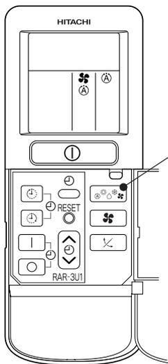
Press the FUNCTION selector so that the display indicates the Ⓐ (AUTO) mode of operation.
