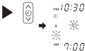
**5** Point the signal window of the remote controller toward the indoor unit, and press the I (RESERVE) button.
