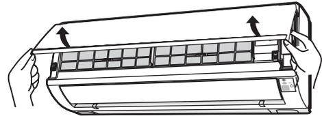
**2** Vacuum dust from the air filter using vacuum cleaner. If there is too much dust, wash the filter with a detergent and rinse it thoroughly. After that, dry it in the shade.
