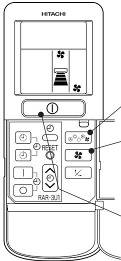
**1** Press the FUNCTION selector so that the display indicates (FAN).
